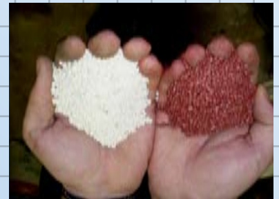
Fast Blending and coating: From ,left to right, at start, a powdered dye is introduced to HIM mixer with granular urea. Five seconds later, the dye is well distributed. At ten seconds total time, the granules are completely encapsulated. At right, before and after photos of same urea.
